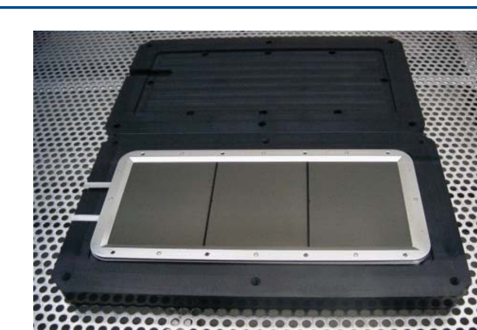
Figure 11: Microchannel plate detector. Positively biased MCP panels detect beam arrival and departure; capture beam position and profile. 160 X 100 mm EGA Array shown.
